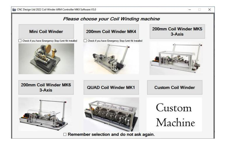
If you have fitted a limit switch on the Mini Coil Winder or the 200mm Coil Winder MK4 then you can tick the checkbox for this option, rather than using the Custom Coil Winder configuration.
