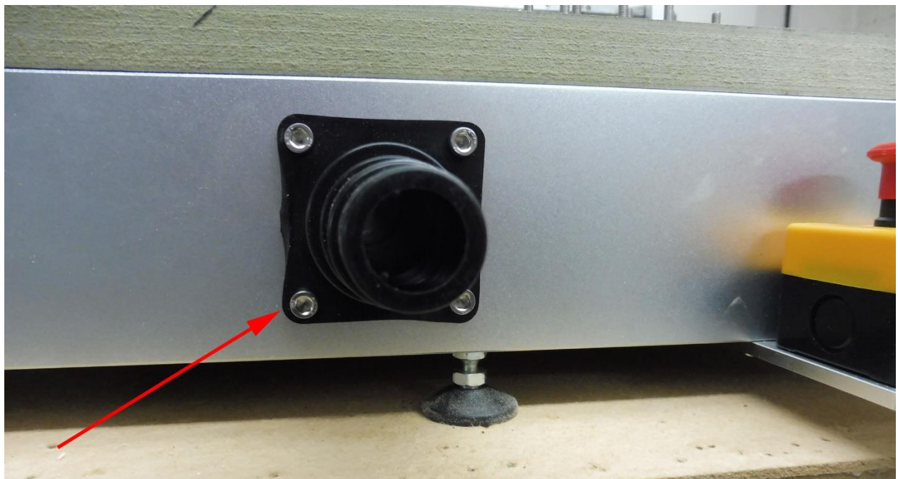
Bolt in the M6 x 16mm screws into the rubber hose adapter.
