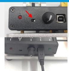
The Power supply comes with an inline power switch. Ensure this is turned off when connecting to the DC power box.
